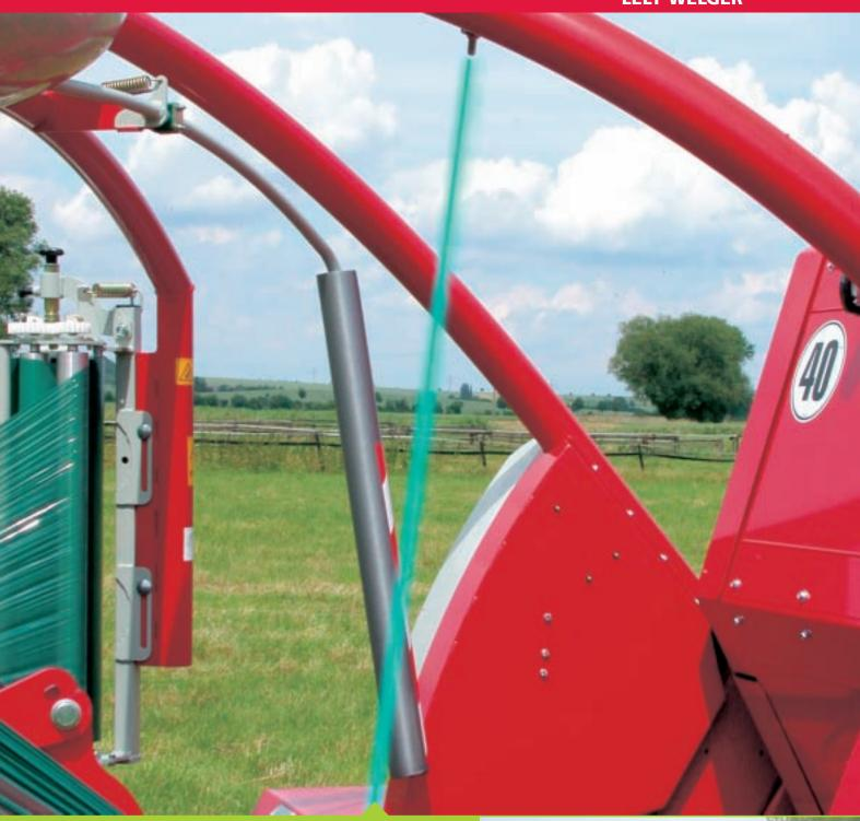
Monitoring of film breakage
